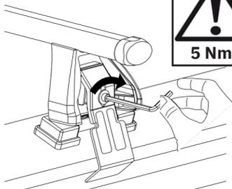
You must regularly check that your roof bars are secured to the correct Nm. We strongly recommend that you check & retighten your roof bars after the initial fitting, after adding & securing a load, before and during your journey.
